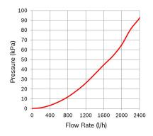
Nominal Voltage (V): 24 Pressure drop (kPa): 45 Flow rate (I/h): 1500 Switchable Pressure difference (kPa): 160 Resistance (Ω): 48
