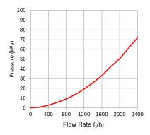
Nominal Voltage (V): 12 Pressure drop (kPa): 45 Flow rate (I/h): 1500 Switchable Pressure difference (kPa): 160 Resistance (Ω): 12,4
