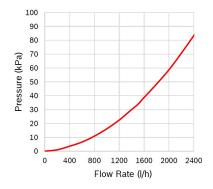
Nominal Voltage (V): 12 Pressure drop (kPa): 35 Flow rate (I/h): 1500 Switchable Pressure difference (kPa): 100 Resistance (Ω): 15,3
