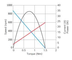
Nominal power (W): 8,6 Nominal current (A): 5 Nominal speed (rpm): 820 Nominal torque (Nm): 0,1 Stall torque (Nm): 1,5 Transmission ratio: 27:4 Hall Sensor: Yes Transmission position: Right
