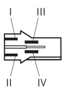
Housing: TE 968182-1 Locker: TE 968183-1 PIN: TE JPT 927768-1 (x2) / Micro-Timer-III 968052-1 (x2)
