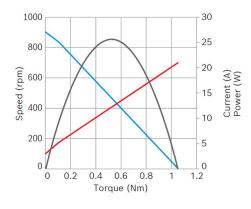
Nominal power (W): 8,8 Nominal current (A): 5 Nominal speed (rpm): 845 Nominal torque (Nm): 0,1 Stall torque (Nm): 1,05 Transmission ratio: 27:4 Hall Sensor: Yes Transmission position: Left
