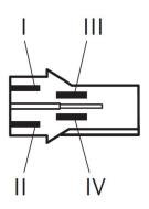
Housing: TE 968183-1 Locker: TE 968182-1 PIN: TE JPT 927768-1 (x2) / Micro-Timer-III 968052-1 (x2)
