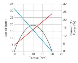
Nominal power (W): 6,1 Nominal current (A): 6 Nominal speed (rpm): 29 Nominal torque (Nm): 2 Stall torque (Nm): 20,5 Transmission ratio: 185,5:1 Hall Sensor: No Transmission position: Right
