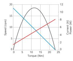
Nominal power (W): 3,5 Nominal current (A): 2 Nominal speed (rpm): 16,9 Nominal torque (Nm): 2 Stall torque (Nm): 23,3 Transmission ratio: 217:1 Hall Sensor: Yes Transmission position: Left
