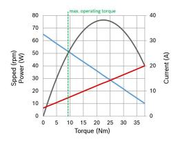
Nominal power (W): 15 Nominal current (A): 7.5 Nominal speed (rpm): 52 Nominal torque (Nm): 9.5 Stall torque (Nm): 38 Transmission ratio: 68:1 Rotation direction: Left and right rotation Hall Sensor: Yes Transmission position: Right
