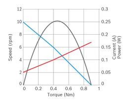
Nominal power (W): 0,3 Nominal current (A): 0,10 Nominal speed (rpm): 6 Nominal torque (Nm): 0,4 Stall torque (Nm): 0,9 Transmission ratio: 405:1 Degree of protection: IP 40 Signal potentiometer: No
